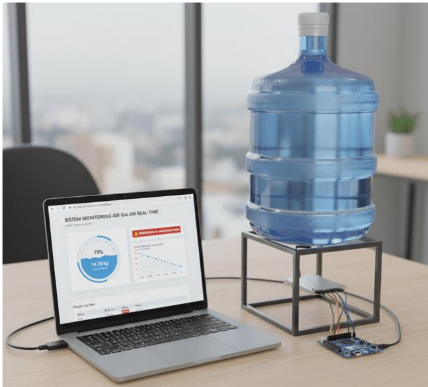
Gambar 4. Visualisasi Implementasi Sistem Monitoring Air Galon Real-Time Berbasis IoT
